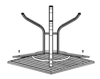
Loosely attach each leg with one bolt and one washer. Do not fully tighten until all four legs are attached.
